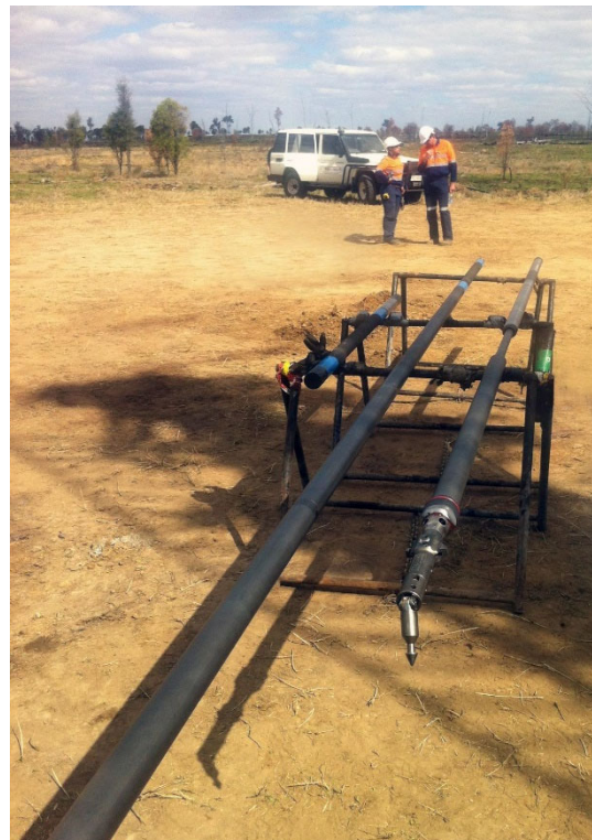
STX60 – CSG Permeability Testing in Queensland (Picture courtesy of Klohn Crippen inc)
