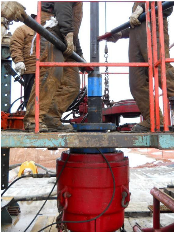
ST114 – Injection Fall Off Testing for a US Government sponsored CO 2 Sequestration Project in Illinois USA
