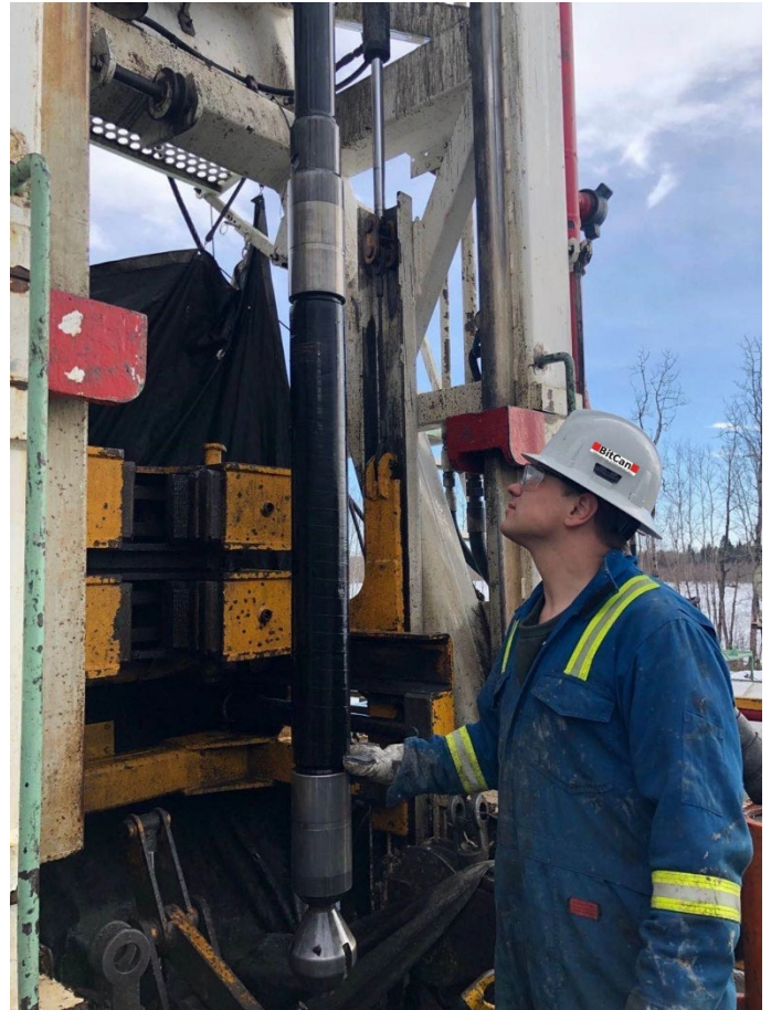
ST114 Minifrac testing in Northern Alberta (Picture courtesy of BitCan inc)
