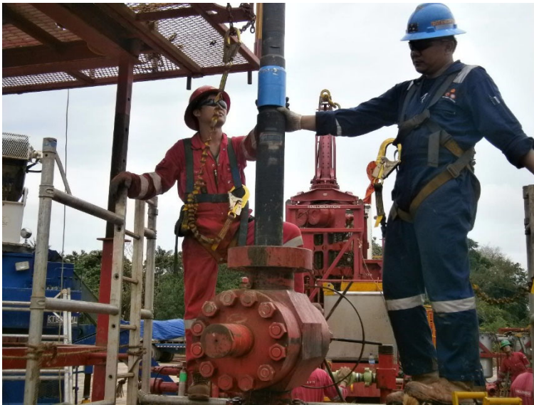
ST114 – Miinifrac testing in Kalimantan using coiled tubing (Picture courtesy of PT Gas Fields Testing)
