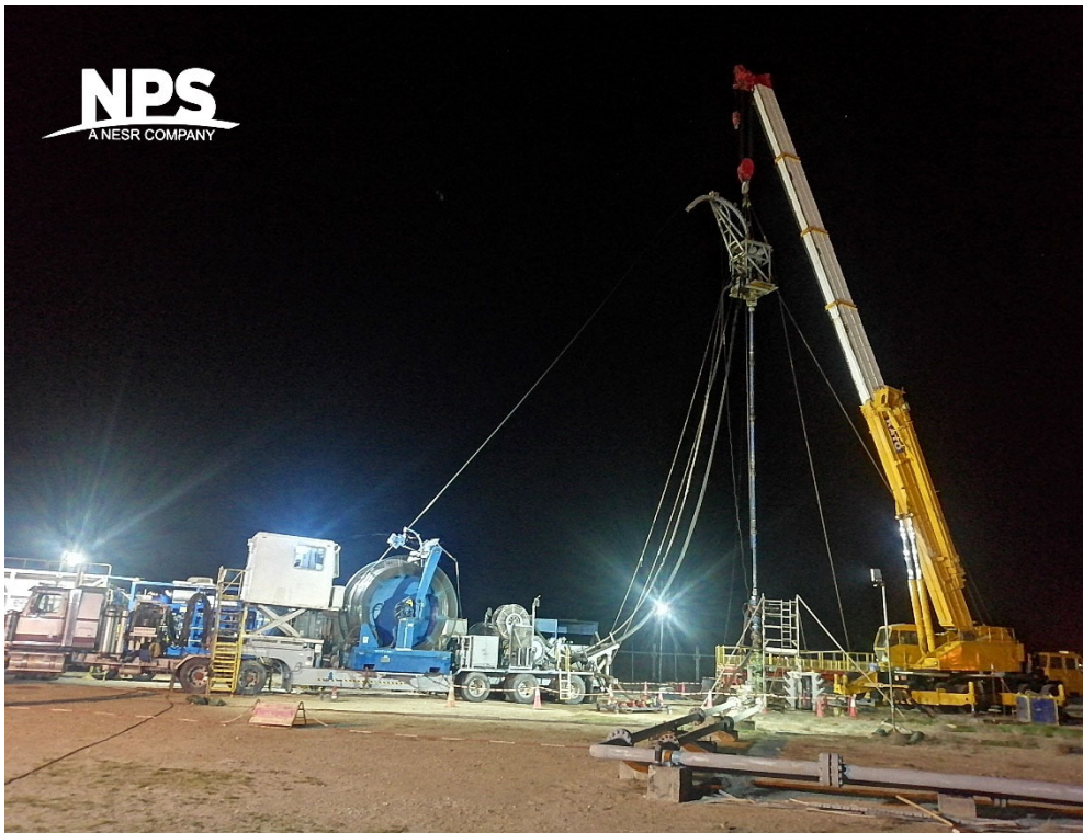
ST60 used for acid frac stimulation (Picture courtesy of National Petroleum Services (NPS), a NESR company)
