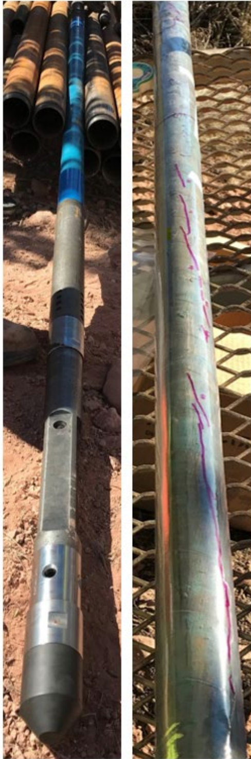
Fig. 4. Left photo showing impression packer (blue section above) combined with core orientation device (bottom) prior to deployment, and right photo showing the transfer of fracture traces to film post-deployment.
