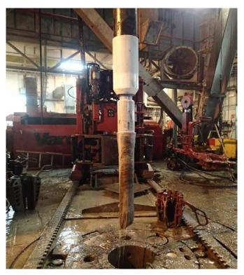
The loss circulation zones intersected during drilling were successfully plugged using the RCP. The RCP was deflated and retrieved. The photo below shows a parted 1.5m stump of fibre glass tubing below the packer (the first of three successful jobs). The plastic shroud below the packer stayed in place. The packer was set at a MD of 3500m (TVD 1400m). The packer system is simple to use and was operated by the rig crew.
