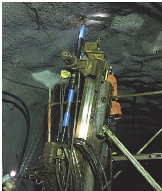
Figure 2 Hydrofracture for preconditioning using a straddle packer assembly
