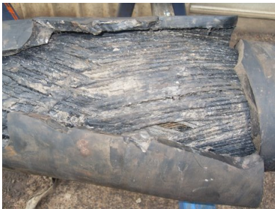
Failed oilfield type packer
