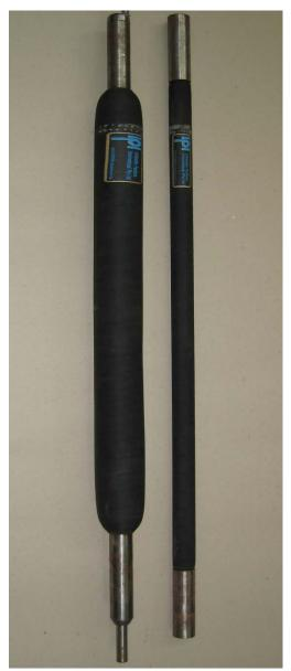
Inflatable Packers International Pty Ltd www.inflatable-packers.com Wall thickness for a packer has more to do with the strength of the reinforcement than with the actual rubber thickness. Several types of reinforcement at commonly available:
