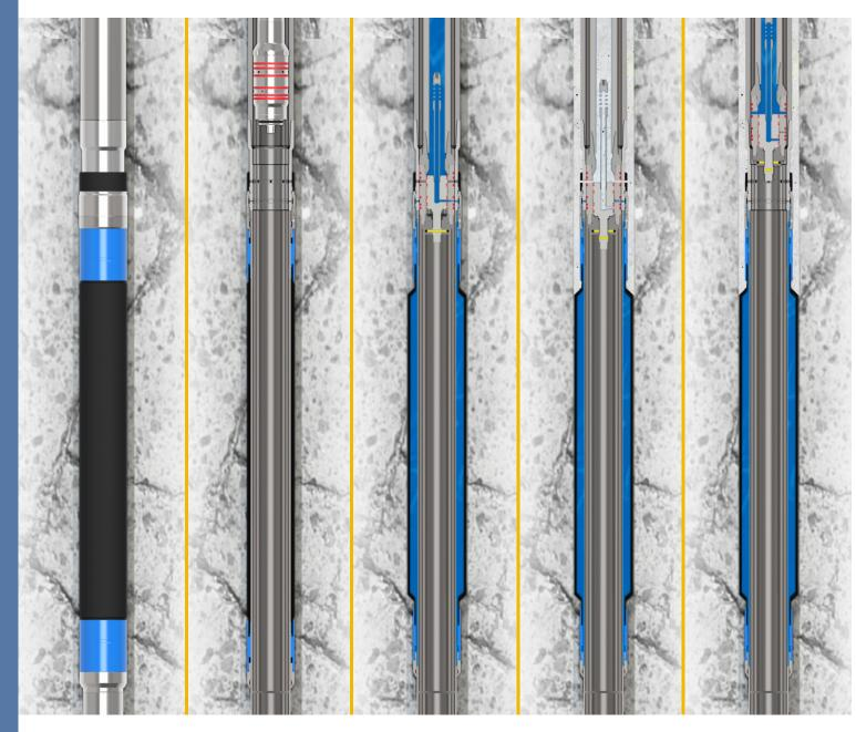
Run In Casing with BHA Run In Setting Tool on pipe to seat in packer Pump water to inflate Packer and shear Setting Tool to cementing position Perform cement job Pull back Setting tool, circulate excess cement and pull out
