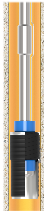
Swage Casing Patch in Three Stages
