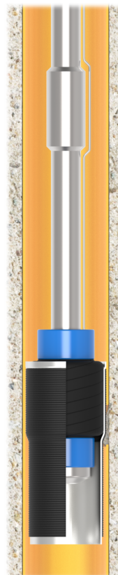
Swage Casing Patch in Three Stages
