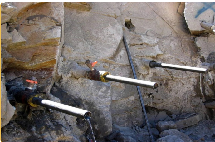
A series of PVC tube mounted pipe packers for a copper mine's tailing dam.
